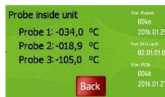
Shows the temperature of the probes inside the unit and the software versions of the Display, SD card and PCB.
