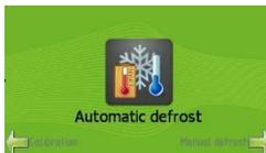
Set the time between automatic defrost cycles on the unit.
