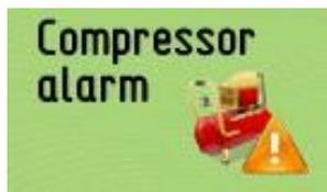
The Compressor failure alarm indicates that a compressor on unit is malfunctioning. When Compressor alarm occurs, the controller switch off the specific Compressor relay, for protecting the Compressor to prevent too high current.
