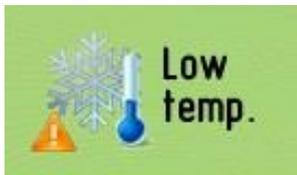
The Low temperature alarm indicates that the temperature of the unit is lower than permitted in the settings of the unit.
