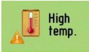
The High temperature alarm indicates that the temperature of the unit is higher than permitted in the settings of the unit.
