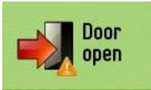
The Door open alarm indicates that the door has not been closed correctly.
