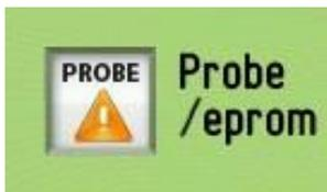
The Probe/Eprom failure alarm indicates that the probe is not working correctly.
