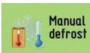
The Manual defrost status indicates that a manually activated defrost cycle is running.
